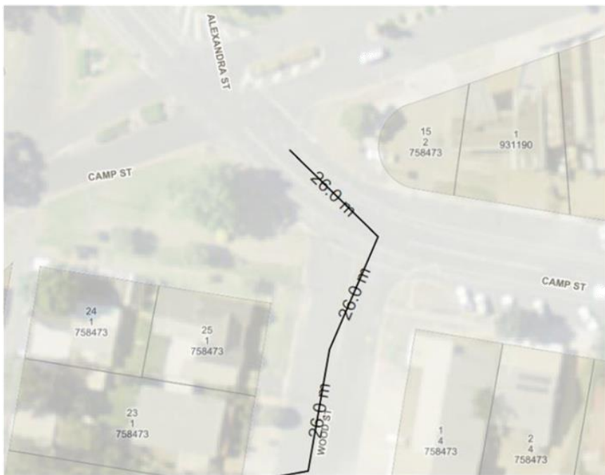
Figure 2: Approximate manoeuvre path of a heavy vehicle (B-double) intercepting the proposed No Parking location
