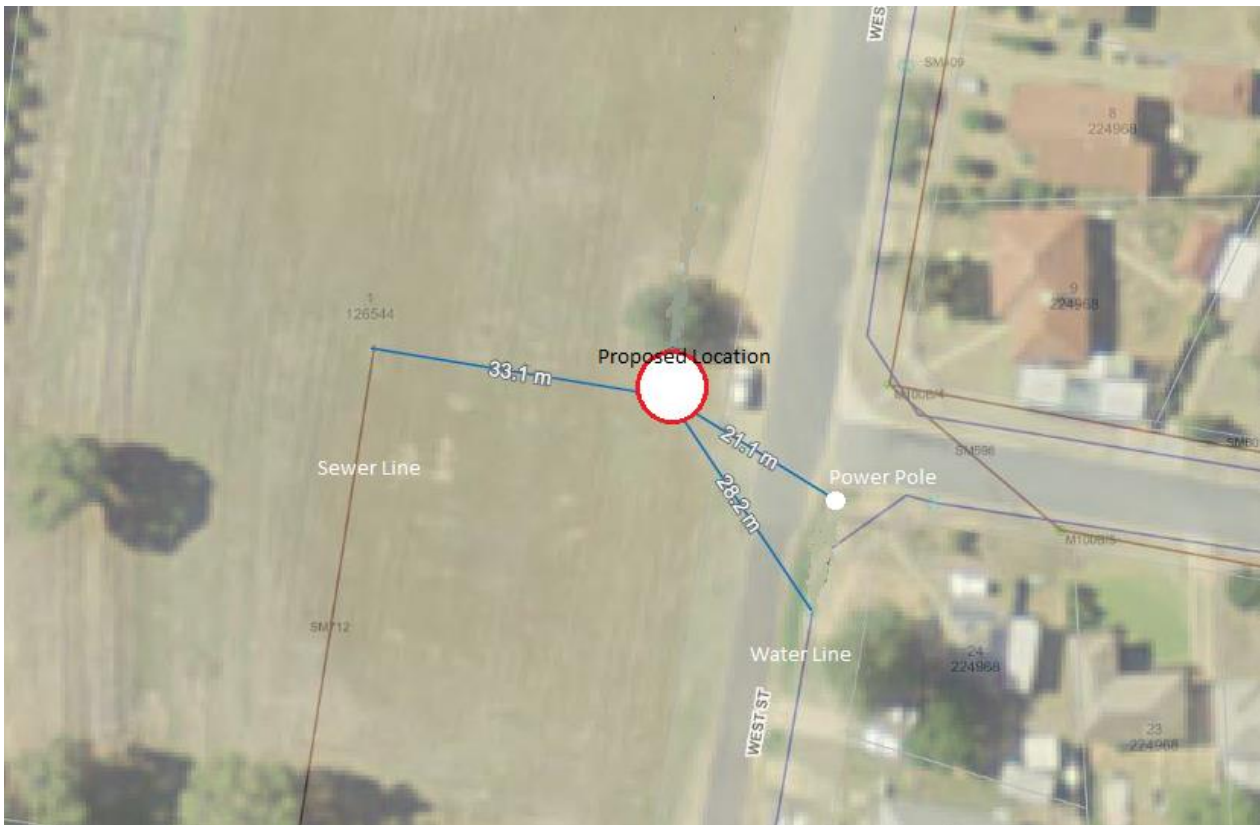
Figure 1: Proposed location of amenities at the dog park and its distances from utilities
