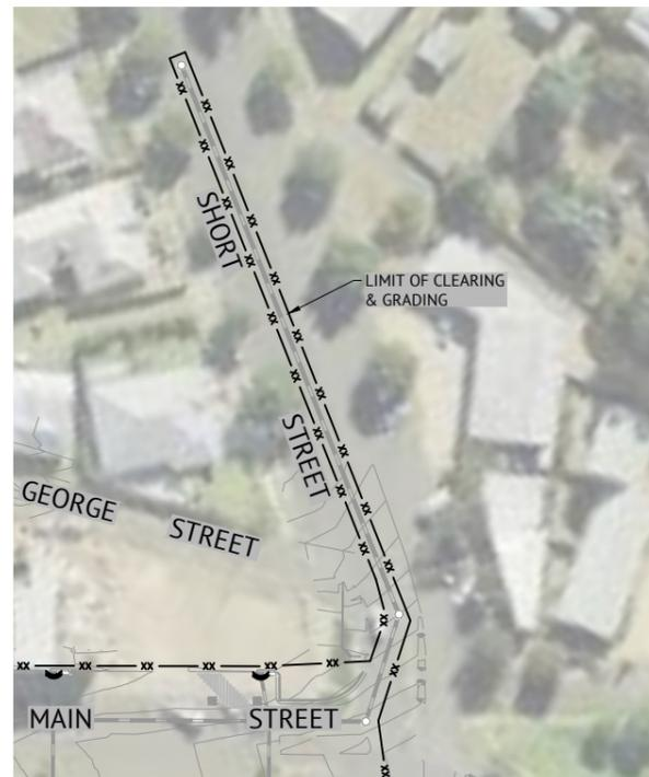
**SHORT STREET EROSION AND SEDIMENT CONTROL DETAIL**
