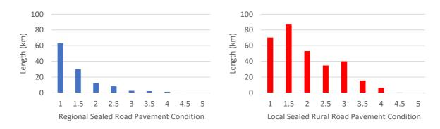
As can be seen, there is very little pavement in poor condition on the regional road network (only 370m in condition 4.5 and 1.4km in condition 4) and little more on the local road network (only 6.6km in condition 4 and 710m in condition 4.5 and 5).
